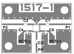
PCB SIZE=19.4x14.0mm PCB: FR-4, t=0.2mm CAPACITOR: size 1005 STRIPLINE WIDTH=0.4mm
