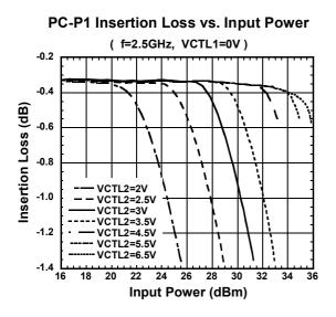
PC-P1 Insertion Loss vs. Input Power
