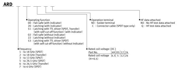
Notes: 1. Sealed types also available, please consult our sales office. (SPDT only) 2. Packing style symbol "Q" is not marked on the relay. 3. 4.5 V DC is failsafe latching only, 5 V DC is TTL drive latching only.
