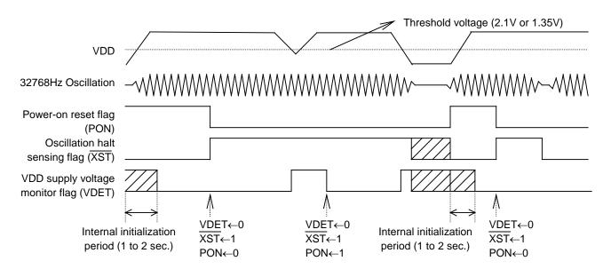
When the PON bit is set to 1 in the control register 2, the DEV, F6 to F0, WALE, DALE,  $\overline{12}$  /24, SCRATCH2, TEST, CT2, CT1, CT0, VDSL, VDET, SCRATCH1, CTFG, WAFG, and DAFG bits are reset to 0 in the oscillation adjustment register, the control register 1, and the control register 2. The PON bit is also set to 1 at power-on from 0 volts.
