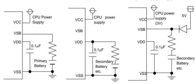
Example of primary battery : CR2032(220mAh), CR1216(30mAh)
