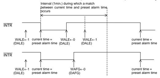
After setting WALE(DALE) to 0, Alarm registers is set to current time, and WALE(DALE) is set to 1, INTR will be not driven to "L" immediately, INTR will be driven to "L" at next alarm setting time.
