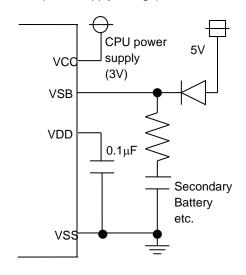
VDD pin cannot be connected to any additional heavy load components such as SRAM. And VDD pin must be connected C2, and C2 should be over  $0.1\mu F$ .
