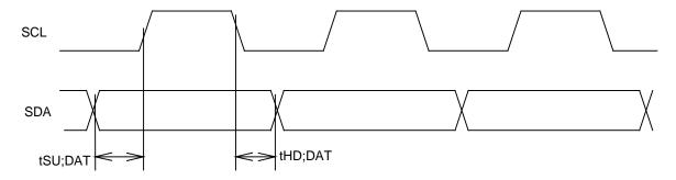
The SCL and SDA pins are at the "H" level when no data transmission is made. Changing the SDA from "H" to "L" when the SCL and the SDA are "H" activates the Start Condition and access is started. Changing the SDA from "L" to "H" when the SCL is "H" activates Stop Condition and accessing stopped. Generation of Start and Stop Conditions are always made by the master (see the figure below).
