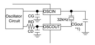
\*1) The CGout should have a capacitance ranging from 0 to 15 pF.
