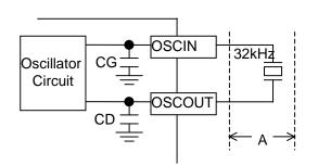
Typical externally-equipped element  $\begin{array}{c} \hbox{X'tal}: 32.768 \hbox{kHz} \\ \hbox{(R1=30k}\Omega \ \hbox{typ)} \\ \hbox{(CL=6pF to 8pF)} \end{array}$  Standard values of internal elements  $\hbox{CG,CD 10pF} \quad \hbox{typ}$
