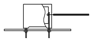
Temperature monitored inside the capacitor.
