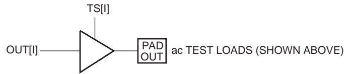
Figure 74. ac Test Loads
