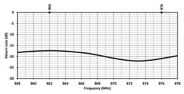
Figure 3. ANT-868-MHW Antenna Return Loss
