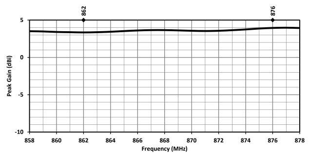
Figure 4. ANT-868-MHW Antenna Peak Gain
