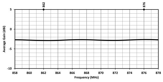
Figure 5. ANT-868-MHW Antenna Average Gain
