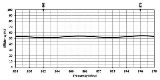
Figure 6. ANT-868-MHW Antenna Radiation Efficiency
