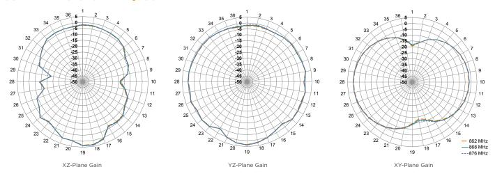
Figure 7. Radiation Patterns for ANT-868-MHW Antenna
