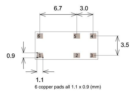
\*CAD files of the antenna footprint are available at www.antenova-com.
