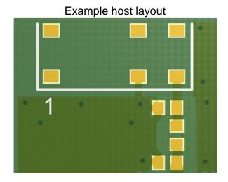
Below shows the antenna footprint and clearance through all layers on the PCB. Only the antenna pads and connections to feed and GND are present within the antenna area
