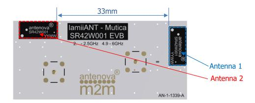
Two antennas placed perpendicular to each other. Both antennas were optimised and matched for the same bands using the Antenova evaluation PCB. An S21 measurement between these antennas shows good isolation of <15dB minimum.
