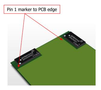
The antenna requires a copper clearance on all PCB layers under the antenna section. The clear-out area is defined below. The clearance is minimal but must be followed for the antenna to function correctly.
