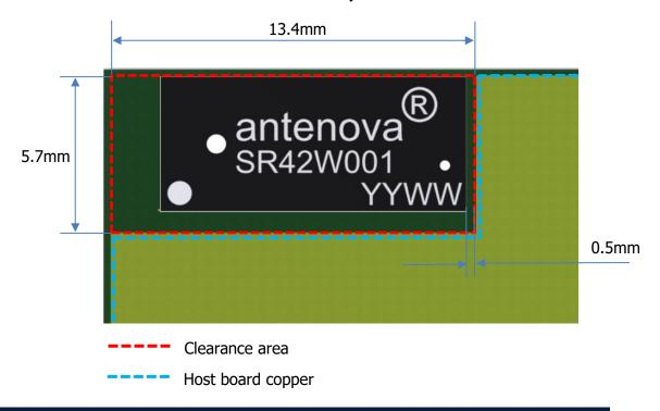
For locations that are not on the corner the following clearances are required from each side of the antenna to GND.
