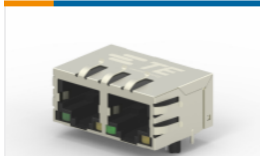
TE Part #2301996-8 RJ45 JACK INT. MAG. 1GB LED 1X2
