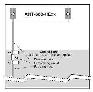
Figure 9. 868-HE Series Antenna Recommended Layout.
