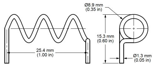
Figure 1. 868-HESM Antenna Dimensions
