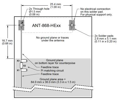
Figure 11. 868-HE Series Antenna Placement on PCB.
