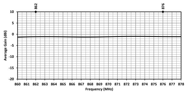
Figure 6. 868-HE Series Antenna Average Gain
