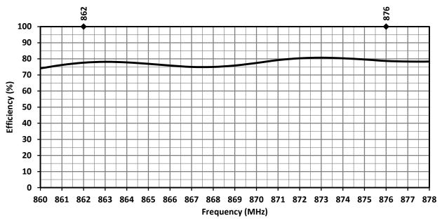
Figure 7. 868-HE Series Antenna Radiation Efficiency
