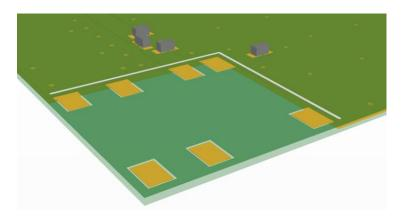
The clear-out area is simply defined as the same size as the antenna. No additional clearance is required.
