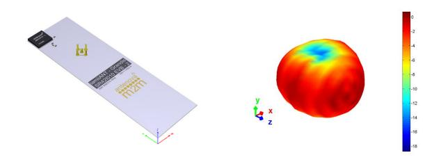
**3D pattern at 915 MHz**Drag to rotate pattern and PCB by using Adobe Reader
