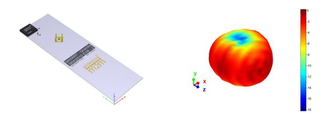
**3D pattern at 867 MHz**Drag to rotate pattern and PCB by using Adobe Reader
