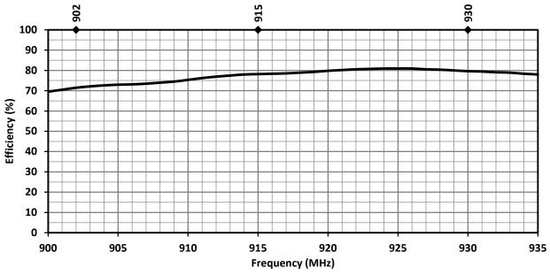
Figure 15. ANT-915-IPW1-RPS Antenna Radiation Efficiency, Straight
