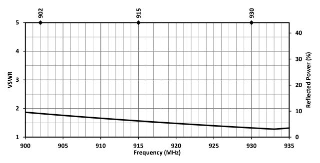
Figure 4. ANT-915-IPW1-RPS Antenna VSWR, Edge Bent
