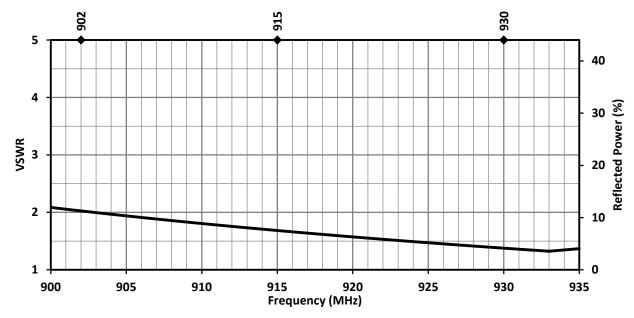
Figure 11. ANT-915-IPW1-RPS Antenna VSWR, Straight
