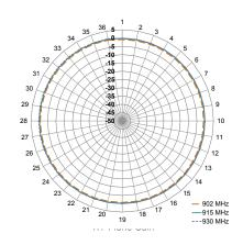
Figure 16. Radiation Patterns for ANT-915-IPW1-RPS, Straight
