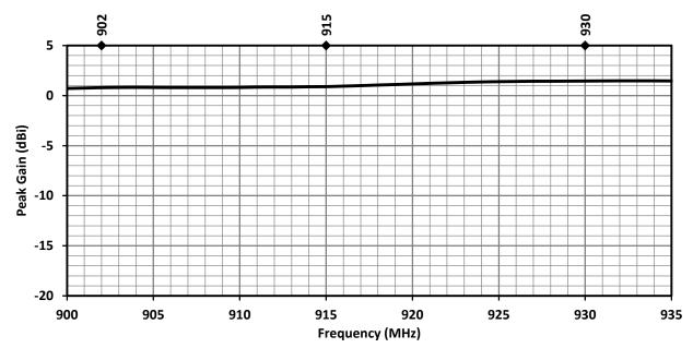
Figure 13. ANT-915-IPW1-RPS Antenna Peak Gain, Straight
