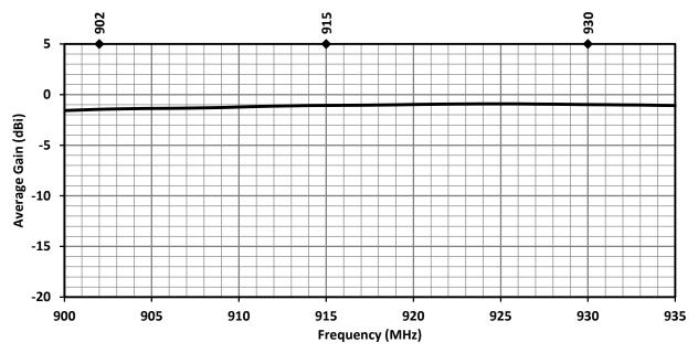
Figure 14. ANT-915-IPW1-RPS Antenna Average Gain, Straight
