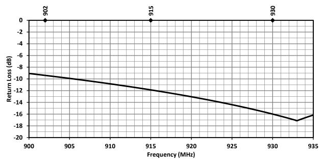
Figure 12. ANT-915-IPW1-RPS Antenna Return Loss, Straight
