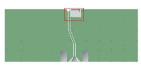
PCB size : 50mm x 20mm x 1mm Antenna area : 8 x 5 mm
