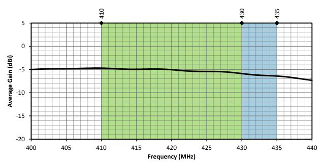
Figure 5. ANT-433-SPS1 Antenna Average Gain with Frequency Band Highlights
