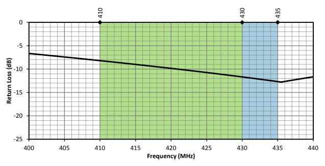
Figure 3. ANT-433-SPS1 Antenna Return Loss with Frequency Band Highlights
