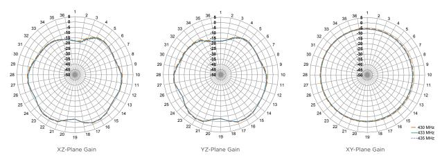
Figure 7. Radiation Patterns for ANT-433-SPS1 Antenna
