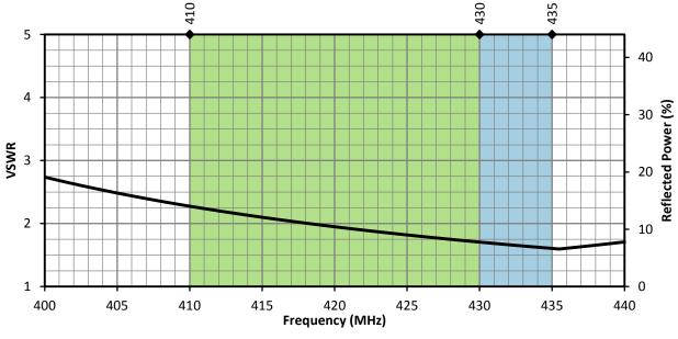
Figure 2. ANT-433-SPS1 Antenna VSWR with Frequency Band Highlights
