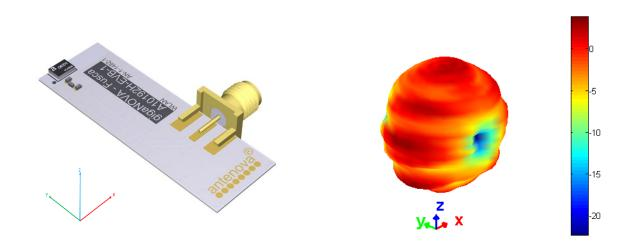
**3D pattern at 2450 MHz**Drag to rotate pattern and PCB by using Adobe Reader
