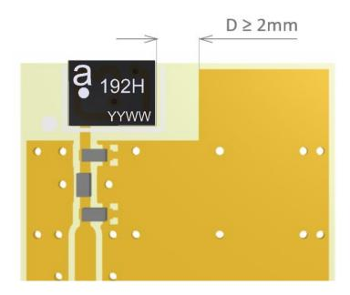
Additional ground and components near the antenna should be at a distance of at least 2 mm. Where possible the antenna should be clear of ground from both sides, although the antenna can work well with a minimum clearance of  $D \ge 2$  mm as shown in the drawing above.
