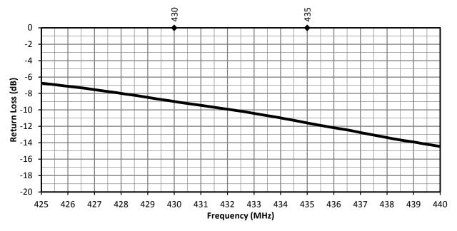
Figure 4. ANT-433-OC-LG Return Loss
