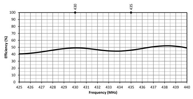
Figure 7. ANT-433-OC-LG Antenna Efficiency
