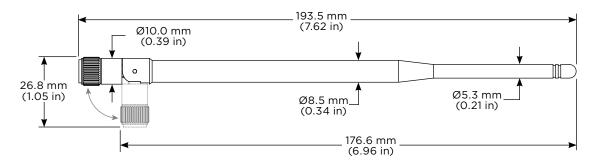
Figure 1. OC-LG Antenna Dimensions
