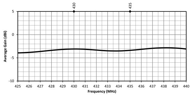
Figure 6. ANT-433-OC-LG Antenna Average Gain
