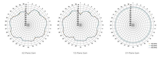
Figure 8. ANT-433-OC-LG Radiation Patterns
