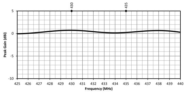
Figure 5. ANT-433-OC-LG Peak Gain
