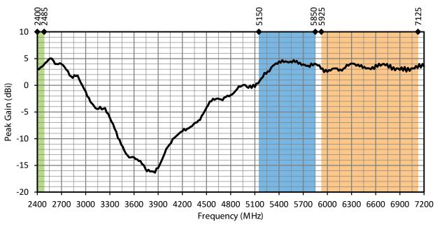
Figure 14: ANT-DB1-WRT-ccc Peak Gain, at Center of Ground Plane
