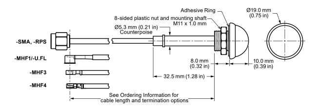
Figure 1: ANT-DB1-WRT Antenna Dimensions
