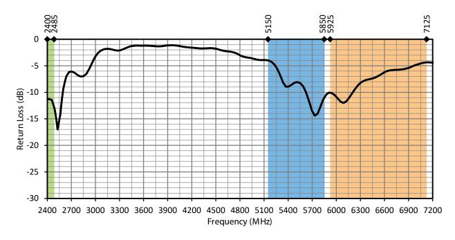
Figure 13: ANT-DB1-WRT-ccc Return Loss, at Center of Ground Plane
