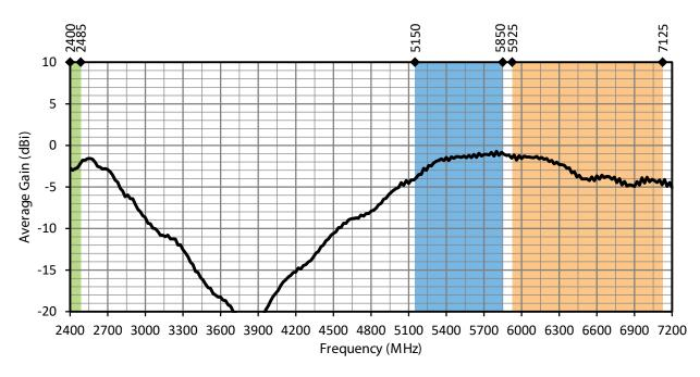
Figure 15: ANT-DB1-WRT-ccc Average Gain, at Center of Ground Plane
