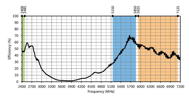
Figure 9: ANT-DB1-WRT-ccc Radiation Efficiency, Free Space
