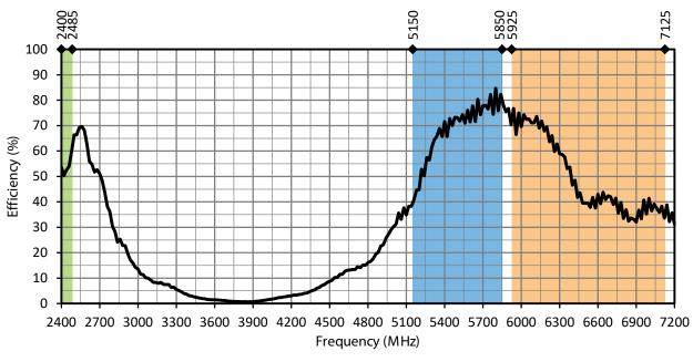
Figure 16: ANT-DB1-WRT-ccc Radiation Efficiency, at Center of Ground Plane
