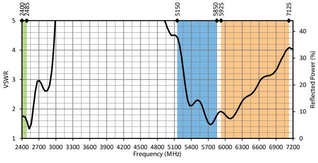
Figure 12: ANT-DB1-WRT-ccc VSWR, at Center of Ground Plane
