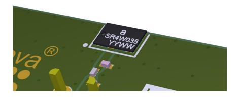
Where the centre is not a viable option, the antenna can be placed offset on the PCB to within the limits shown below. A minimum of 6mm from either PCB edge should be observed. Where possible this distance should be greater than 6mm.
