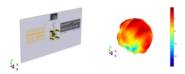
**3D pattern at 2.45 GHz**Drag to rotate pattern and PCB by using Adobe Reader
