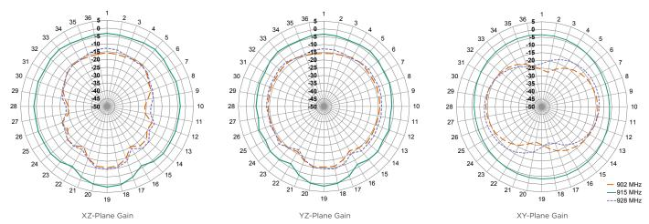
Figure 6. Radiation Patterns for 915-CPA Antenna
