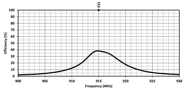
Figure 5. 915-CPA Antenna Radiation Efficiency
