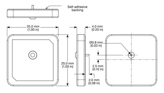
Figure 1. 915-CPA Antenna Dimensions
