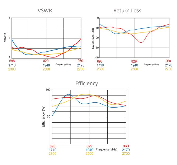
Data measured in free space and on plastic device enclosure
