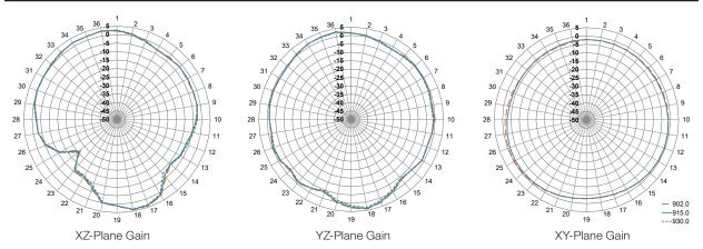
Figure 8. ANT-916-CW-RCL Radiation Patterns
