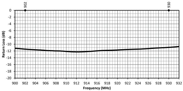
Figure 4. ANT-916-CW-RCL Return Loss
