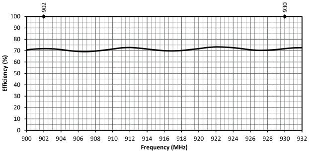
Figure 7. ANT-916-CW-RCL Antenna Radiation Efficiency
