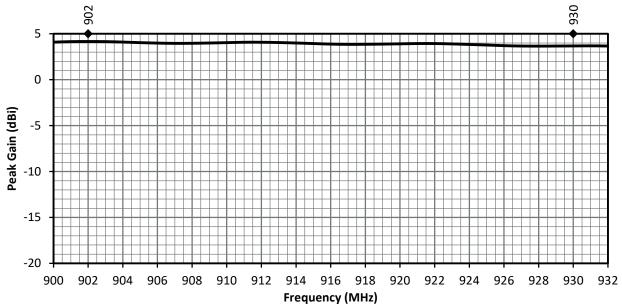
Figure 5. ANT-916-CW-RCL Peak Gain
