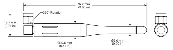
Figure 1. ANT-916-CW-RCL Antenna Dimensions
