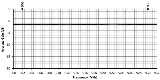
Figure 6. ANT-916-CW-RCL Antenna Average Gain
