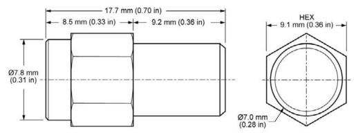
Figure 1. ANT-915-NUB-ccc Antenna Dimensions
