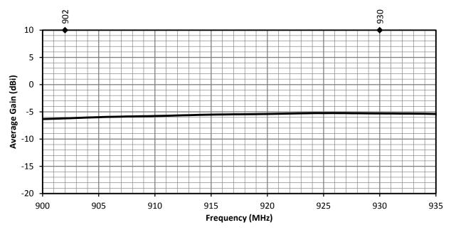
Figure 14. Antenna Average Gain for ANT-915-NUB-ccc Antenna in Free Space
