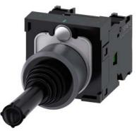
Coordinate switch, 22 mm, round, plastic with metal front ring, black, 2 switch positions, vertical latching, without mechanical interlocking, in O position, with holder, 1 NO, 1 NO, screw terminal, with laser labeling, upper case and lower case, always upper case at beginning of line
