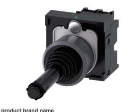
Coordinate switch, 22 mm, round, plastic with metal front ring, black, 2 switch positions, vertical, momentary contact type, with mechanical interlocking in O position, with holder, 1 NO, 1 NO, screw terminal
