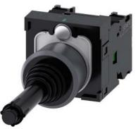
Coordinate switch, 22 mm, round, plastic with metal front ring, black, 2 switch positions, vertical, momentary contact type, with mechanical interlocking in O position, with holder, 1 NO, 1 NO, screw terminal, with laser labeling, upper case and lower case, always upper case at beginning of line
