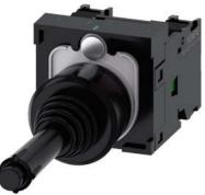
Coordinate switch, 22 mm, round, plastic, black, 2 switch positions, vertical, momentary contact type, with mechanical interlocking in O position, with holder, 1 NO, 1 NO, screw terminal, with laser labeling, upper case and lower case, always upper case at the beginning of the word
