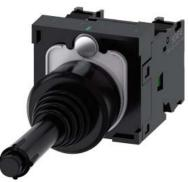
Coordinate switch, 22 mm, round, plastic, black, 2 switch positions, vertical, momentary contact type, with mechanical interlocking in O position, with holder, 1 NO, 1 NO, screw terminal, with laser labeling, upper case
