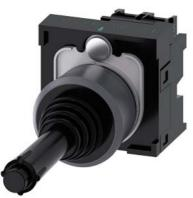
Coordinate switch, 22 mm, round, plastic with metal front ring, black, 2 switch positions, vertical, momentary contact type, with mechanical interlocking in O position, with holder, 1 NO, 1 NO, screw terminal, Z=20-unit packaging
