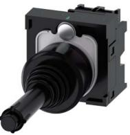
Coordinate switch, 22 mm, round, plastic, black, 2 switch positions, vertical, momentary contact type, with mechanical interlocking in O position, with holder, 1 NO, 1 NO, screw terminal, Z=20-unit packaging
