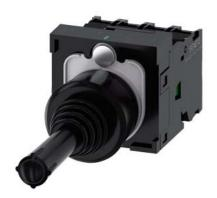
Coordinate switch, 22 mm, round, plastic, black, 4 switch positions, latching, without mechanical interlocking, in O position, with holder, 1 NO, 1 NO, 1 NO, 1 NO, screw terminal, Z=20-unit packaging
