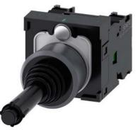
Coordinate switch, 22 mm, round, plastic with metal front ring, black, 2 switch positions, horizontal, momentary contact type, with mechanical interlocking in O position, with holder, 1 NO, 1 NO, screw terminal, with laser labeling, upper case and lower case, always upper case at the beginning of the word
