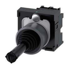
Coordinate switch, 22 mm, round, plastic with metal front ring, black, 2 switch positions, vertical latching, without mechanical interlocking, in O position, with holder, 1 NO, 1 NO, screw terminal, Z=20-unit packaging
