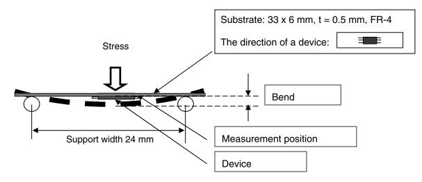
Figure 3. Example of the bend and the rate of distortion Note2
