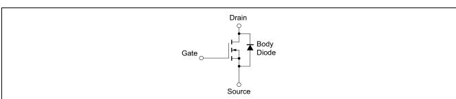
Remark: Strong electric field, when exposed to this device, can cause destruction of the gate oxide and ultimately degrade the device operation. Steps must be taken to stop generation of static electricity as much as possible, and quickly dissipate it once, when it has occurred.
