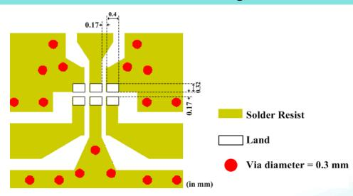
Line width should be designed to match 50 characteristic impedance, depending on PCB material and thickness.
