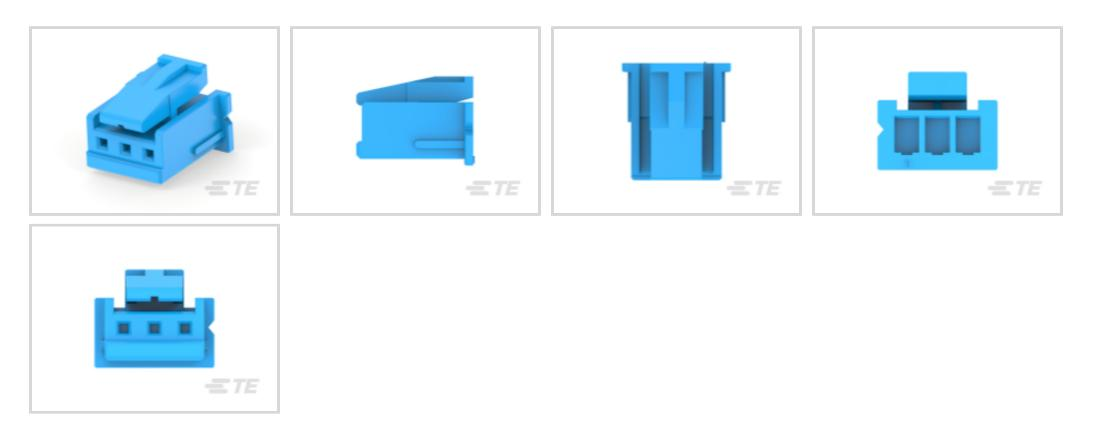
Connector Product Type: Housing Connector & Housing Type: Receptacle Connector System: Wire-to-Board Number of Positions: 3 Centerline (Pitch): 2.5 mm [.098 in ]
