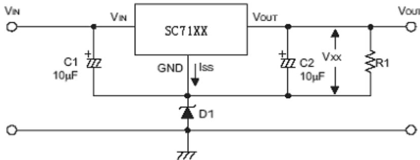
$$V_{OUT} = V_{XX} + VD1$$
