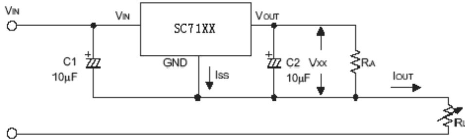
$$I_{OUT} = V_{XX}/R_X + I_{SS}$$
