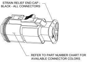
PLUG, 3 SOCKET, AT SERIES, STRAIN RELIEF END CAP
