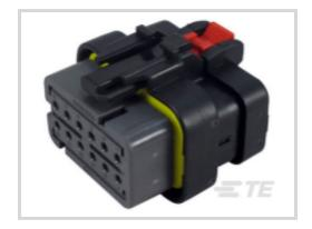
Connector System: Wire-to-Wire Number of Positions: 12 Connector & Housing Type: Housing for Female Terminals Centerline (Pitch): 4.5 mm [.177 in ] Sealable: Yes All AMPSEAL 16 Housings (226)
