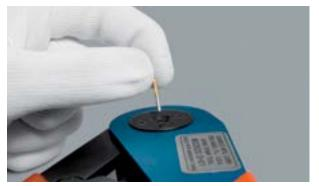
Insert the contact into the crimping tool.
