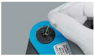
Insert the wire into the contact.
