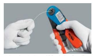
Tighten the crimping tool fully. The handles will not release until the tool is fully bottomed.
