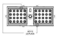
40 POS, PLUG, SOCKET, ARC SERIES, KEYED, RD SEAL, BLACK
