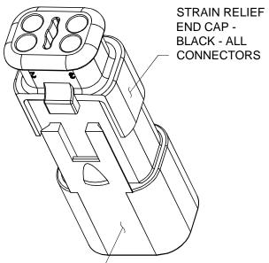
RECEP, 4 PIN, AT, STRAIN RELIEF, REDUCED DIA WIRE SEAL
