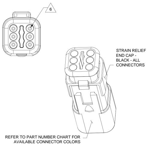
RECEPTACLE, 6 PIN, AT SERIES, STRAIN RELIEF END CAP
