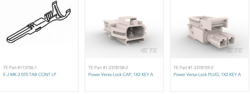
Tab Contact, Tin, 600 VAC, 600 VDC, 26 – 22 AWG Wire Size, .13 – .3 mm<sup>2</sup> Wire Size, Crimp, Brass, Power, Power Versa-Lock 5.0
