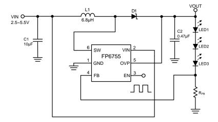
Figure 3. Typical Application Circuit of FP6755 TDFN-6 (2mm×2mm) Package
