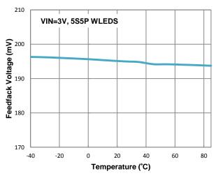
Figure 14. Feedback Voltage vs. Temperature
