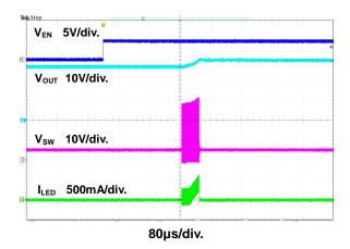
Figure 10. Open Load Protection Waveform
