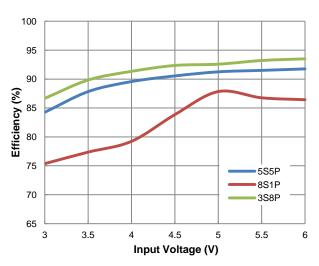
Figure 12. Efficiency vs. Input Voltage
