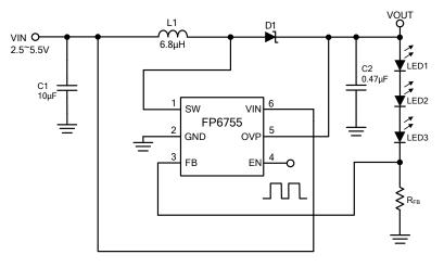
Figure 2. Typical Application Circuit of FP6755 SOT-23-6 Package
