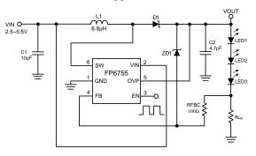
Figure 15. LED Open Circuit Application
