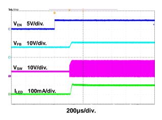
Figure 6. Enable Startup Response Waveform
