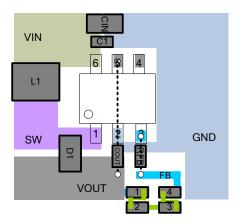
Figure 16. Layout Diagram
