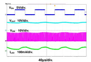
Figure 8. PWM Dimming Response Waveforms at a Frequency of 10kHz
