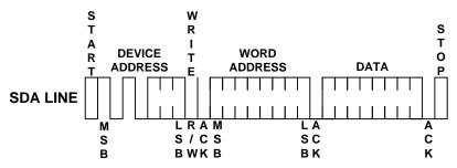
Figure 5: Byte Write
