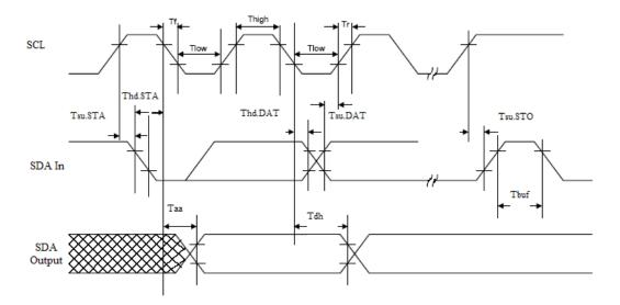
Figure 10: SCL and SDA Bus Timing
