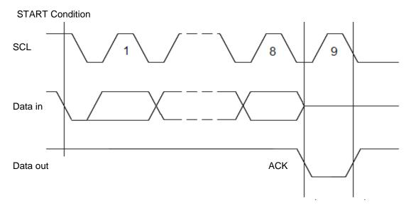
Figure 4: Timing diagram for output ACKNOWLEDGE
