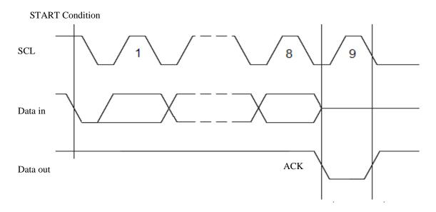
Figure 2: Timing diagram for output ACKNOWLEDGE
