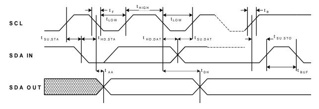
Figure 8: SCL and SDA Bus Timing
