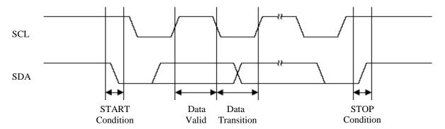
Figure 1: Timing diagram for START and STOP conditions
