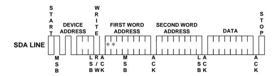
Figure 3: Byte Write
