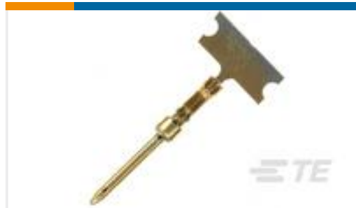
TE Part #1658540-5 CONT,PIN,PLATED,20DF,LP,#24-28
