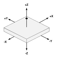
Figure 4. Package Axis Reference
