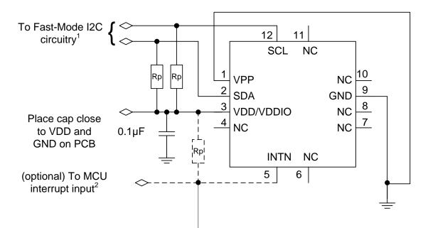
NOTE<sup>1</sup>: Rp are typically 4.7kΩ pullup resistors to VDD/VDDIO, per I2C specification. When pin VDD/VDDIO is powered down, SDA and SCL will be driven low by internal ESD diodes.
