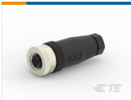
TE Part #T4110501051-000 M12,FEMALE,STRAIGHT,D CODE,5P, PG7,GOLD
