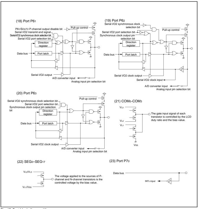
Fig. 17 Port block diagram (4)
