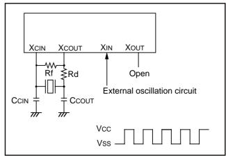
Fig. 60 External clock input circuit
