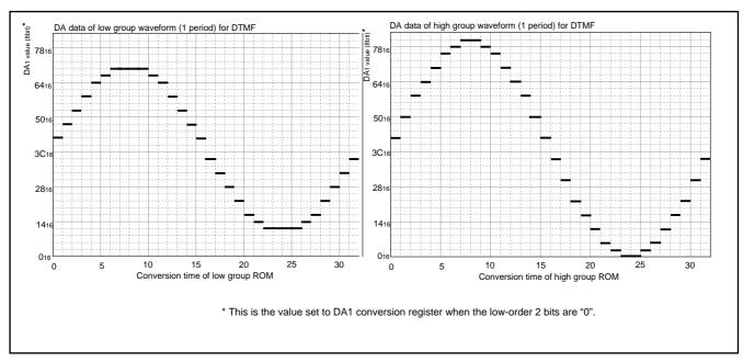
Fig. 43 Waveform data of high group and low group
