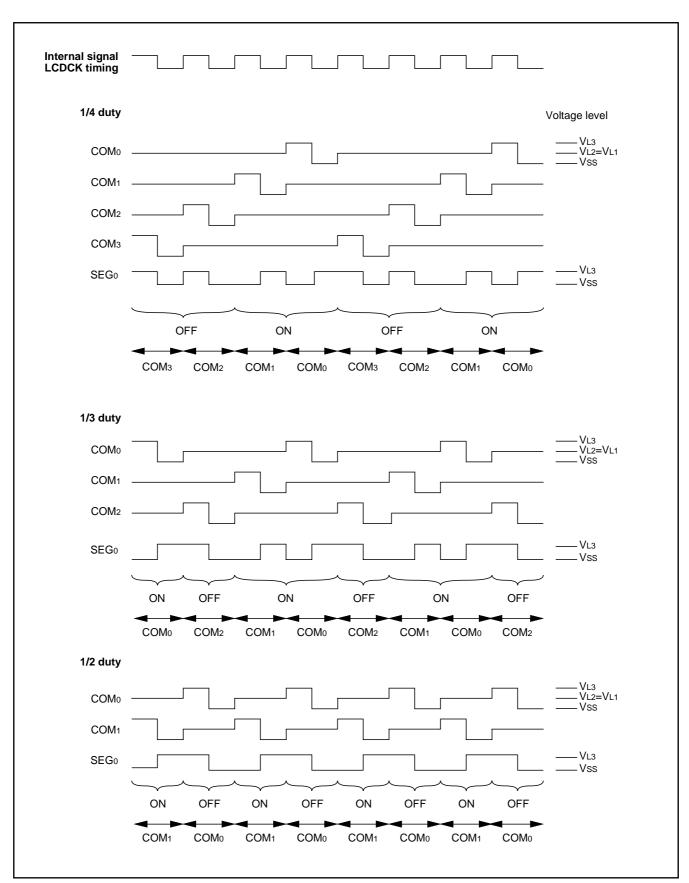
Fig. 50 LCD drive waveform (1/2 bias)
