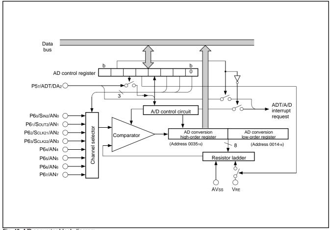
Fig. 40 A/D converter block diagram
