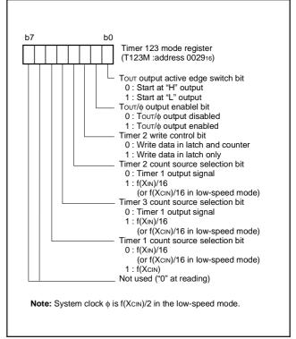
Fig. 25 Structure of timer 123 mode register
