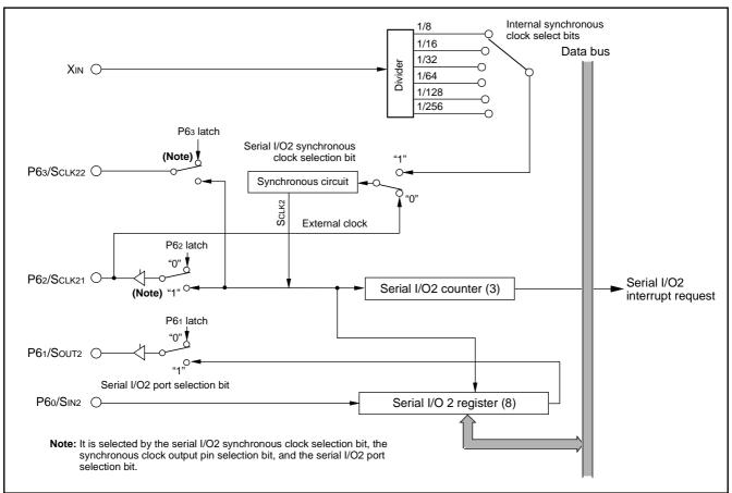
Fig. 32 Block diagram of serial I/O2 function
