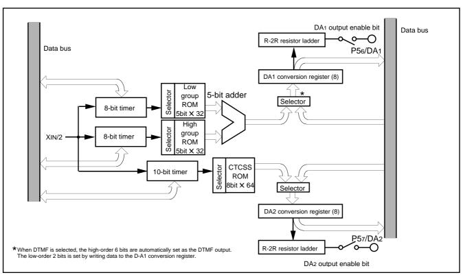
Fig. 42 Block diagram of D/A converter
