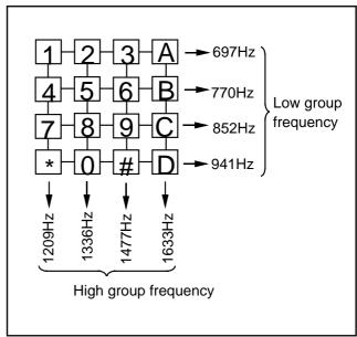
Fig. 44 Key matrix of telephone and rating frequency
