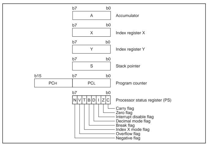
Fig. 6 740 Family CPU register structure
