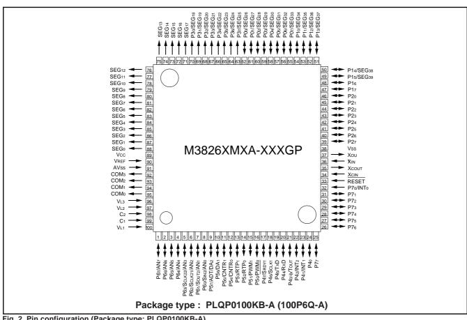
Fig. 2 Pin configuration (Package type: PLQP0100KB-A)
