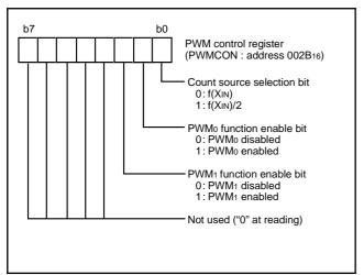
Fig. 36 Structure of PWM control register
