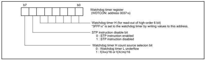
Fig. 53 Structure of watchdog timer control register
