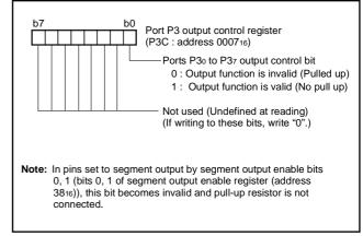
Fig. 12 Structure of port P3 output control register
