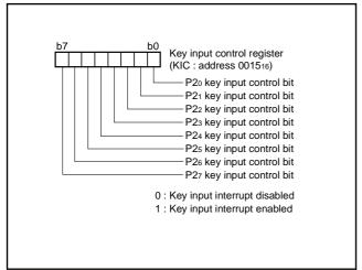
Fig. 21 Structure of key input control register
