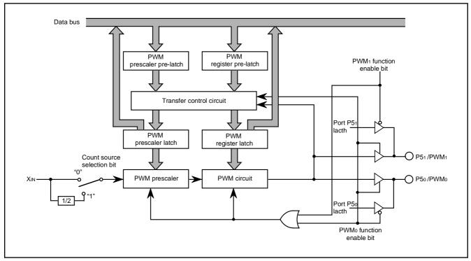
Fig. 35 Block diagram of PWM function
