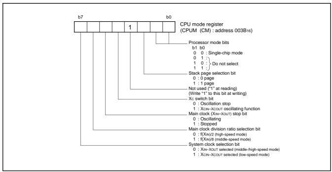
Fig. 8 Structure of CPU mode register
