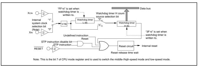
Fig. 52 Block diagram of watchdog timer
