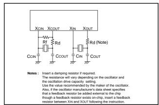
Fig. 59 Oscillator circuit
