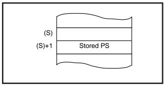
Fig. 3.3.3 Stack memory contents after PHP instruction execution
