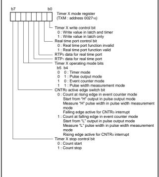
Fig. 23 Structure of timer X mode register
