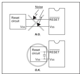
Fig. 63 Wiring for the RESET pin
