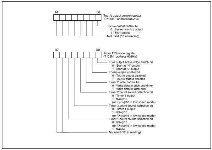
Fig. 55 Structure of Toυτ/φ output-related registers
