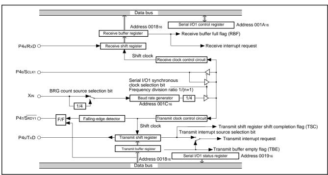
Fig. 26 Block diagram of clock synchronous serial I/O1
