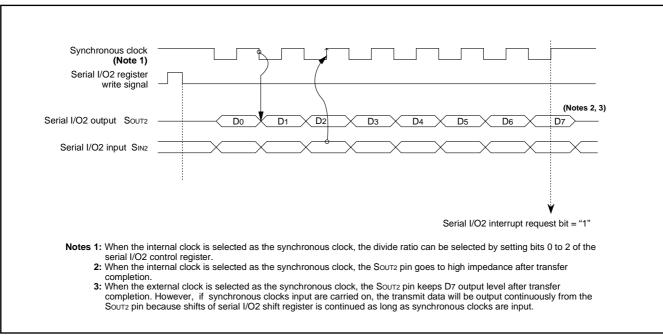
Fig. 33 Timing of serial I/O2 function
