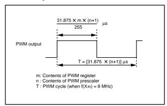
Fig. 34 Timing of PWM cycle
