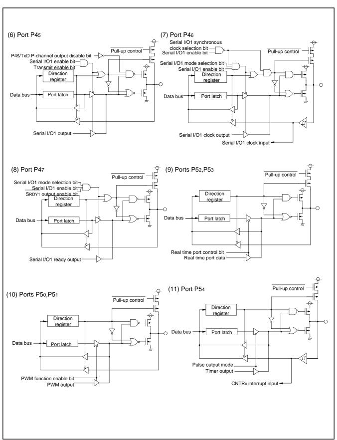
Fig. 15 Port block diagram (2)
