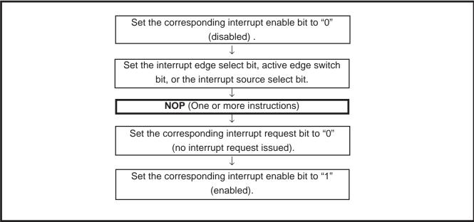
Fig. 3.3.5 Sequence of changing relevant register
