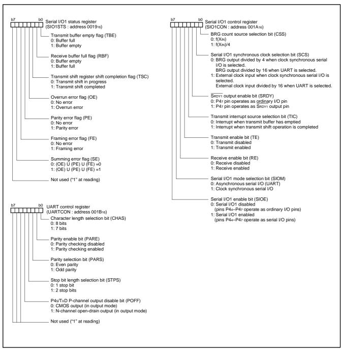
Fig. 30 Structure of serial I/O1 control registers
