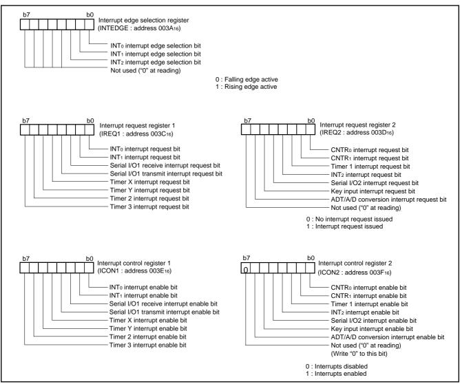
Fig. 19 Structure of interrupt-related registers
