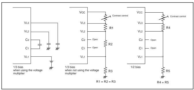
Fig. 48 Example of circuit at each bias
