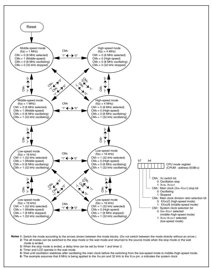
Fig. 62 State transitions of system clock
