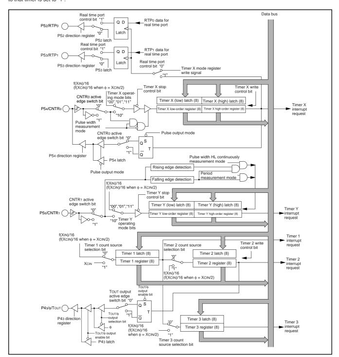
Fig. 22 Timer block diagram
