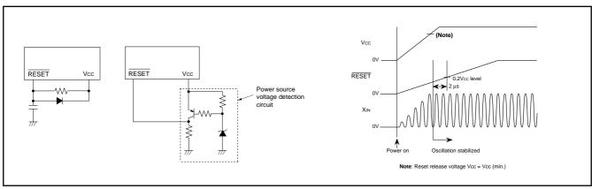
Fig. 56 Example of reset circuit
