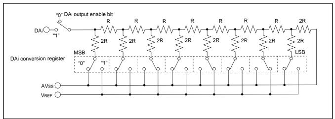
Fig. 45 Equivalent connection circuit of D/A converter
