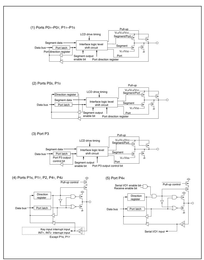
Fig. 14 Port block diagram (1)
