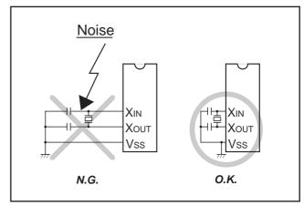
Fig. 64 Wiring for clock I/O pins
