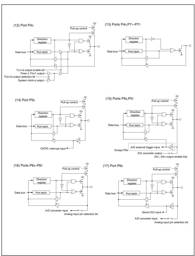
Fig. 16 Port block diagram (3)
