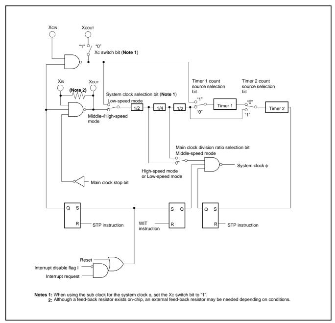
Fig. 61 Clock generating circuit block diagram
