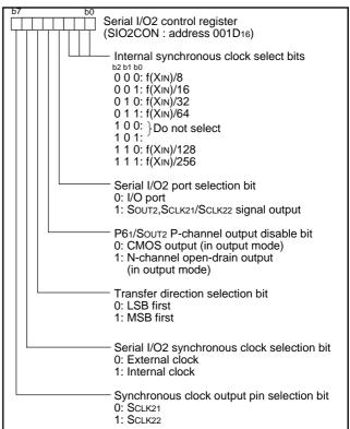
Fig. 31 Structure of serial I/O2 control register
