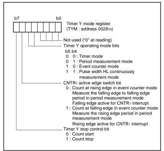
Fig. 24 Structure of timer Y mode register
