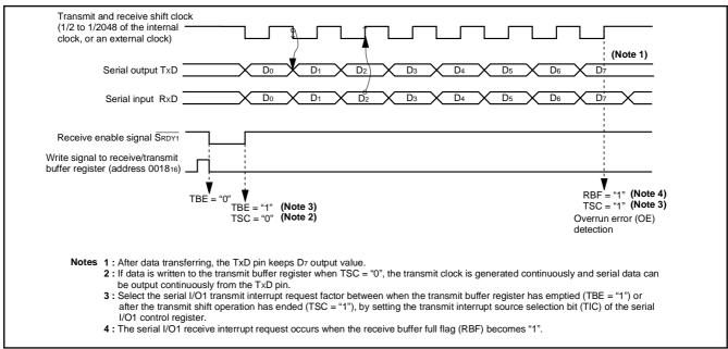
Fig. 27 Operation of clock synchronous serial I/O1 function
