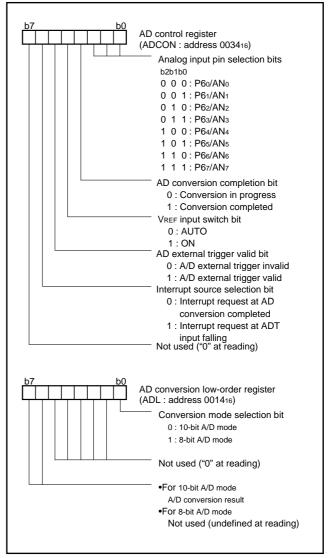
Fig. 38 Structure of A/D converter-related registers
