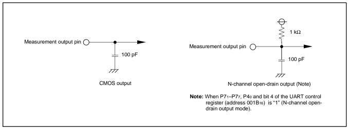
Fig. 65 Circuit for measuring output switching characteristics
