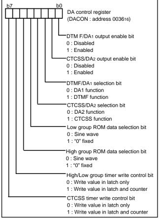
Fig. 41 Structure of DA control register
