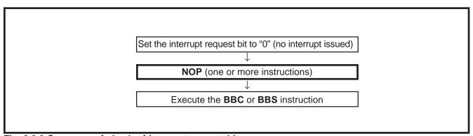
Fig. 3.3.6 Sequence of check of interrupt request bit
