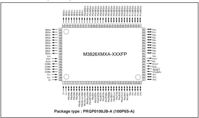
Fig. 1 Pin configuration (Package type: PRQP0100JB-A)
